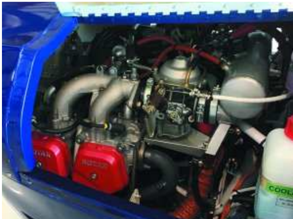
The 115-HP Rotax 912 is the most popular engine option.
