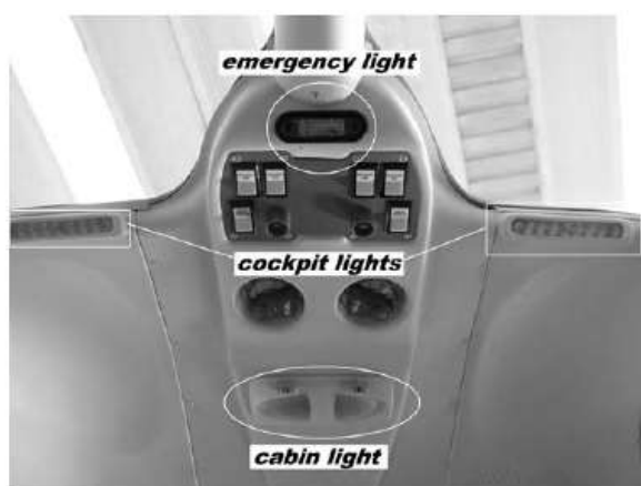
Figure 9. – Over-head panel lights arrangement
