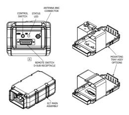
The cockpit-mounted remote switch assembly is comprised of an ELT status LED and control switch, and allows an operator to manually turn the ELT on (i.e., activate) for testing and reset (i.e., deactivate) the ELT.
