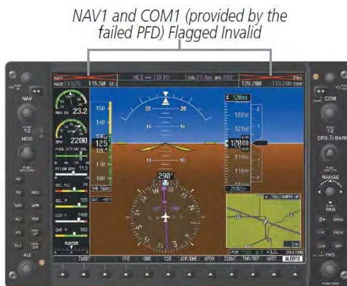
GDU 1044 (MFD) in reversionary mode
