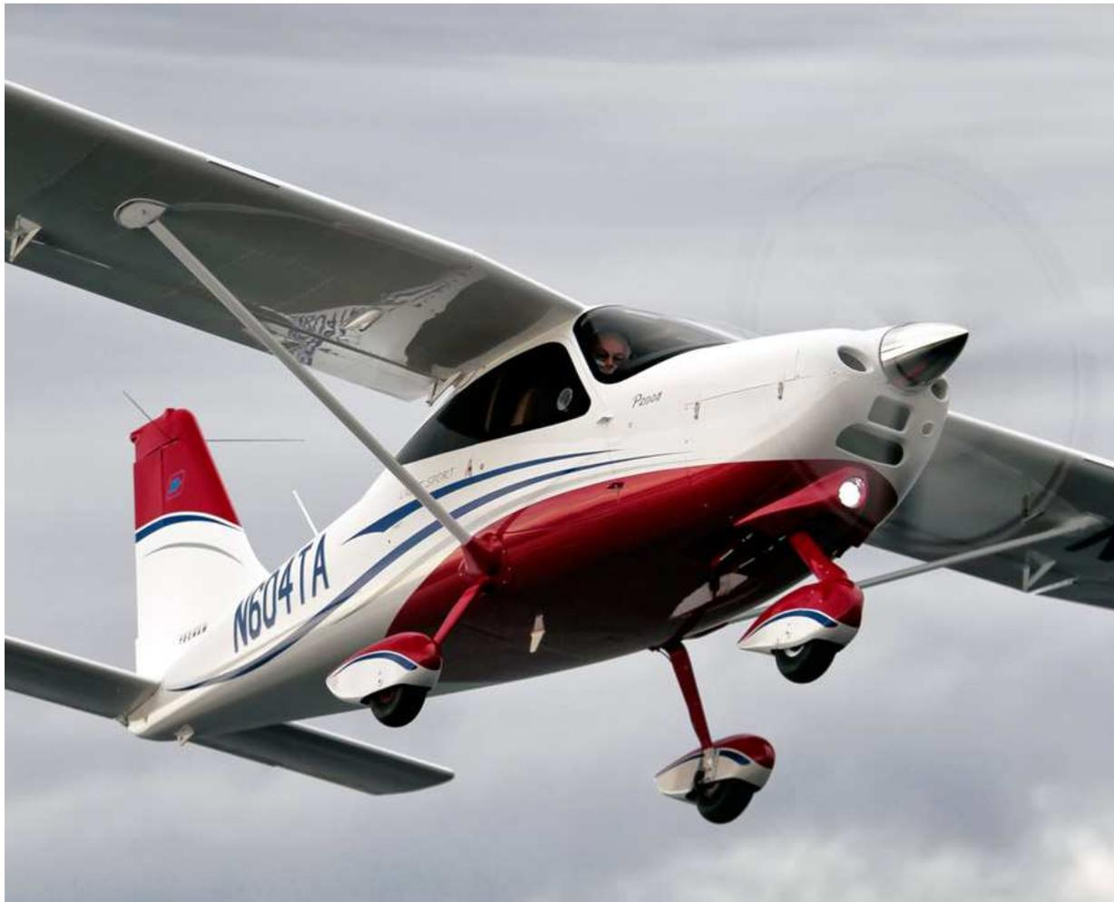
This turbocharged Tecnam P2008 offers several hints of where general aviation may be headed in the future. It brings together less costly construction techniques (metal wings and carbon fiber fuselage) and is certified under less costly rules. On the panel are dramatically less expensive avionics. Some think aircraft like this one may populate flying clubs and rental fleets decades from now, after current four-place, \$400,000 airplanes inflate their way up to \$1 million.
